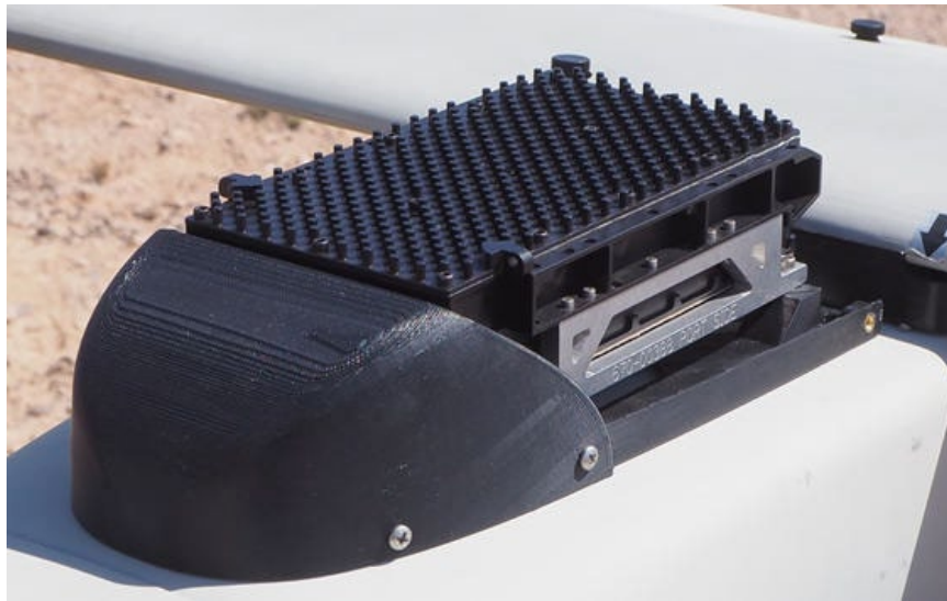
Figure 4-83. Stalker Primary Mount – Payload Installation (3 of 3)
